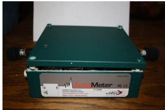
Side View of Frog Logger (Song Meter)
