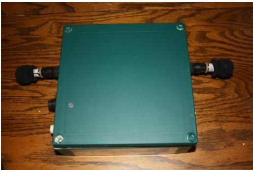
Frog logger with 2 microphones
