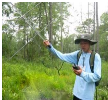
A student using a receiver to find a Box Turtle with a radio transmitter attached.
